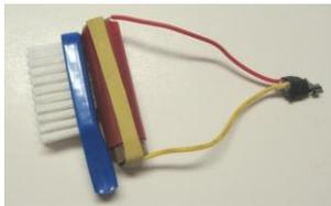
Insert motor wires between rubber band and battery (switch=close the circuit: motor should begin vibrating)
